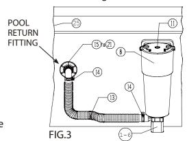
Screws one and a half turns each. Then proceed in tightening them in equal turns each in sequence around the Face Plate until all are equally tight and you have a good even seal. **Warning!** Be sure not to over tighten them, you just need a water tight seal.
